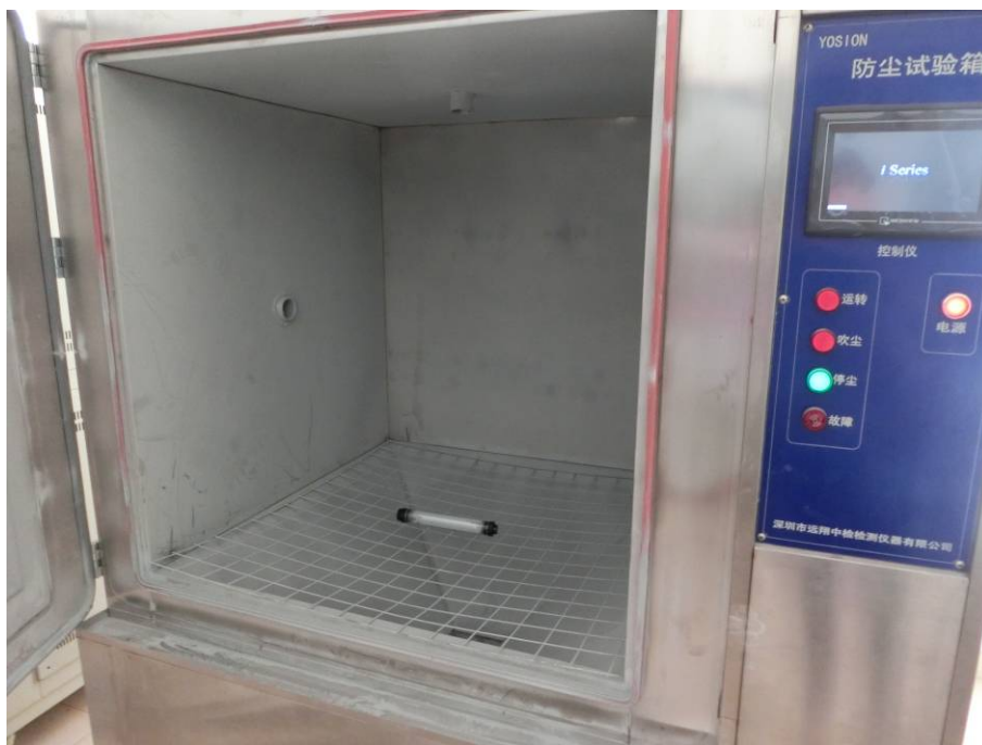
Photo 1 IP 6X test Over View
