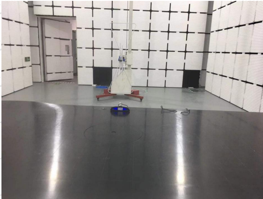
Photo 1 Radiated Emission Test
