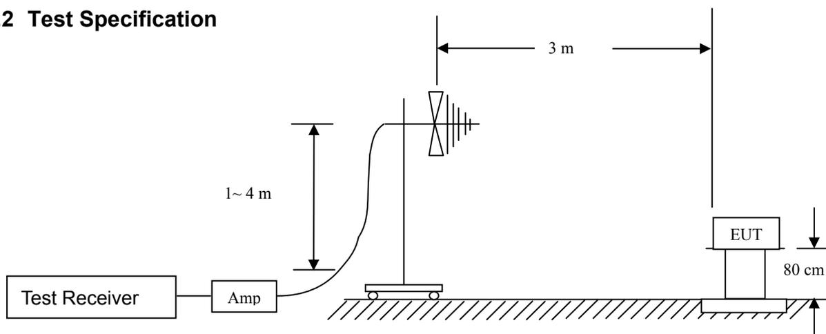
EUT was placed upon a wooden test table which was placed on the turn table 0.8m above the horizontal metal ground plane, and operating in the mode as mentioned above. A receiving antenna was placed 3m away from the EUT. During testing, turn around the turn table and move the antenna from 1m to 4m to find the maximum field-strength reading. All peripherals were placed at a distance of 10cm between each other. Both horizontal and vertical antenna polarities were tested.
