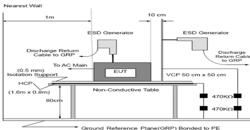
EUT was operated in the mode as mentioned above. Both contact and air discharge was executed. Contact discharge to the conductive surfaces and to coupling planes; air discharge at insulating surfaces. Each test point shall be subjected to 10 discharges at least (For each voltage and polarity).
