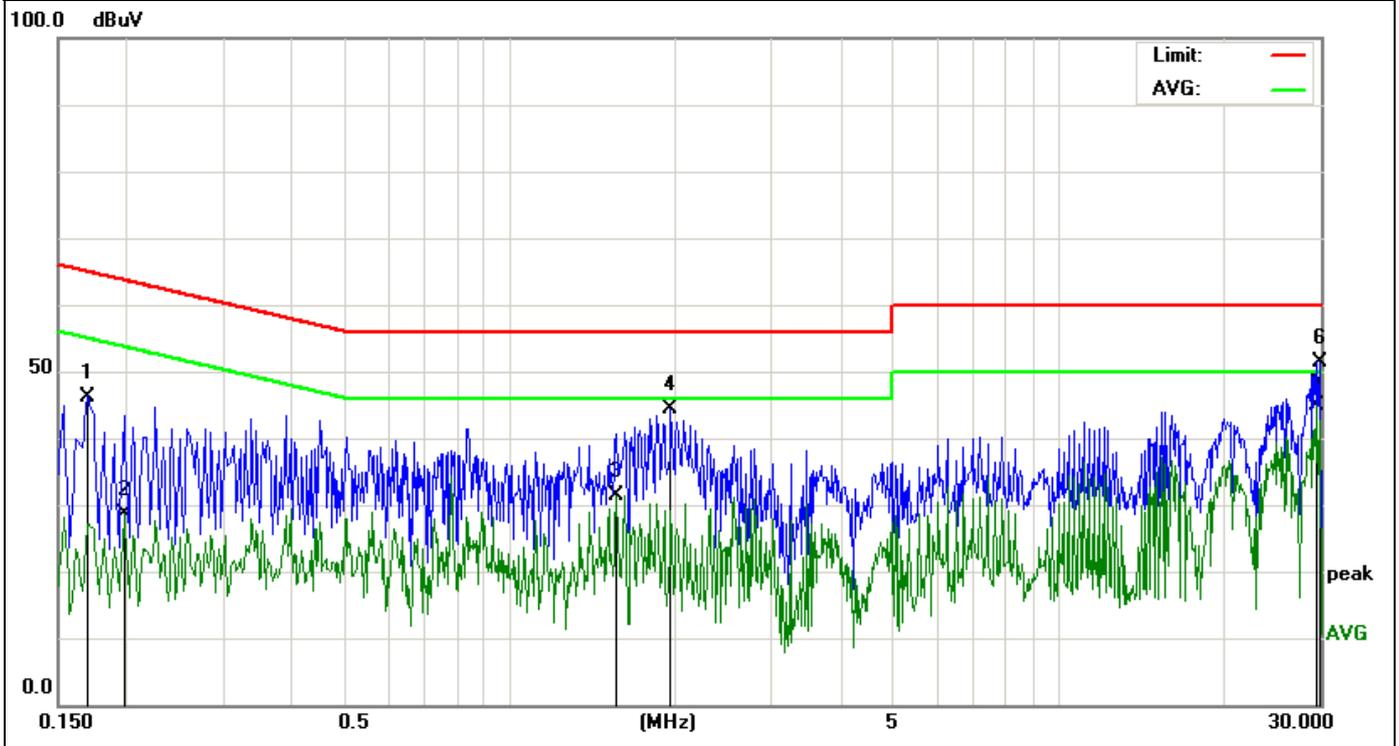
Remark: Correct Factor = LISN factor + Cable Loss + Pulse limiter factor.
