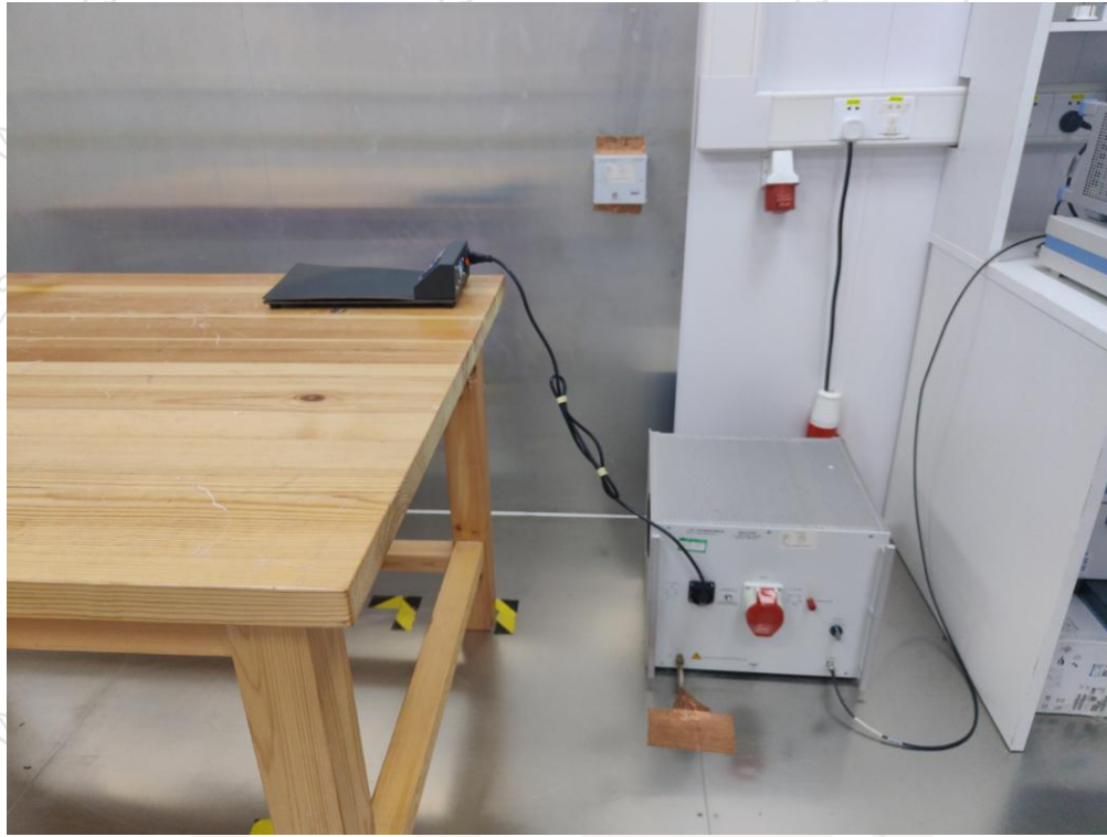
Setup for Conducted Emission
