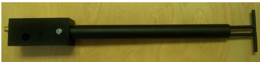
Figure 1 – MVG COMOSAR Validation Dipole
