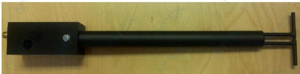
Figure 1 – MVG COMOSAR Validation Dipole
