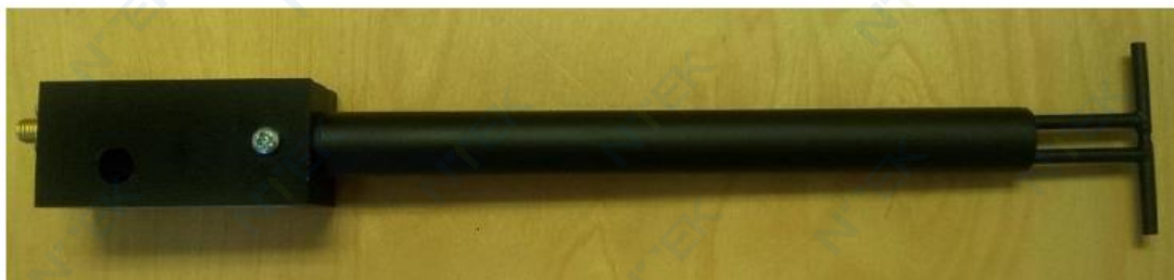
Figure 1 – MVG COMOSAR Validation Dipole
