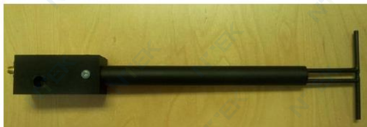
Figure 1 – MVG COMOSAR Validation Dipole
