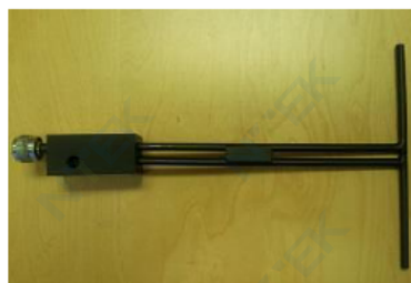
Figure 1 – MVG COMOSAR Validation Dipole
