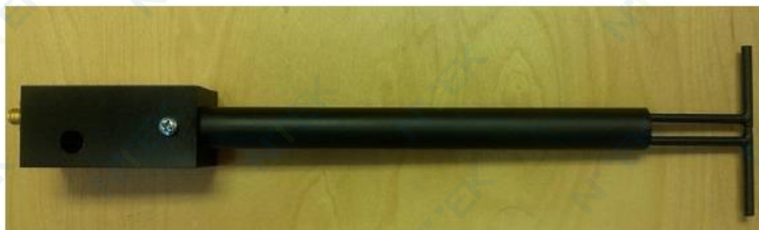
Figure 1 – MVG COMOSAR Validation Dipole
