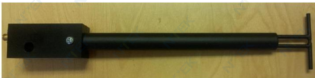
Figure 1 – MVG COMOSAR Validation Dipole
