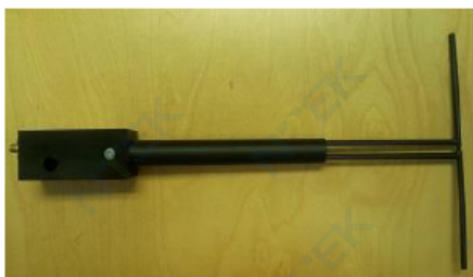
Figure 1 – MVG COMOSAR Validation Dipole
