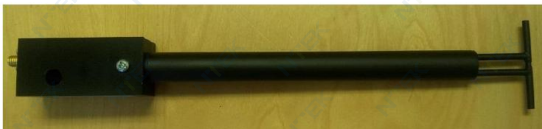
Figure 1 – MVG COMOSAR Validation Dipole
