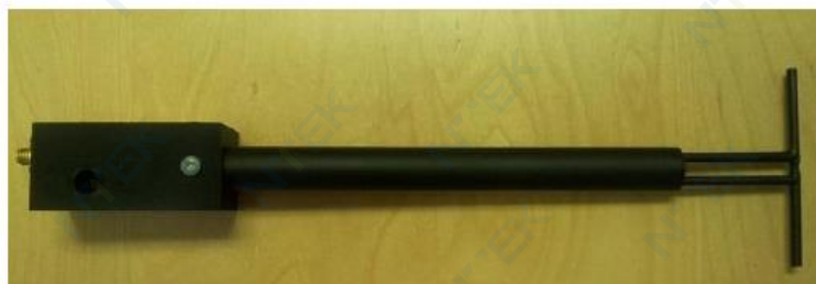
Figure 1 – MVG COMOSAR Validation Dipole
