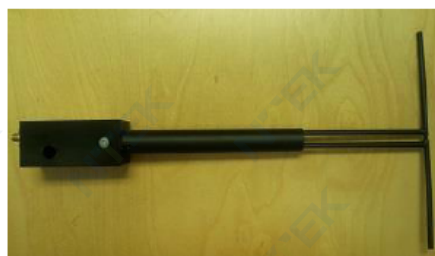
Figure 1 – MVG COMOSAR Validation Dipole
