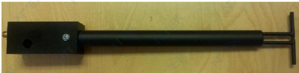
Figure 1 – MVG COMOSAR Validation Dipole
