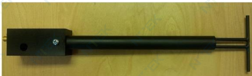
Figure 1 – MVG COMOSAR Validation Dipole
