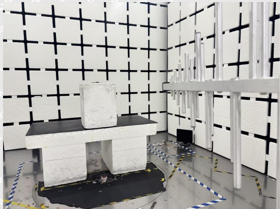
Spurious Emission Test Setup (Below 1GHz)
