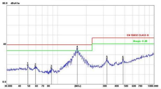
Site LAB Limit: EN 55032 CLASS B Polarization: Horizontal
