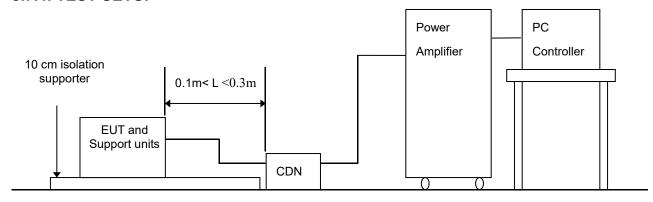
Note: 1. The EUT is setup 0.1m above Ground Reference Plane
