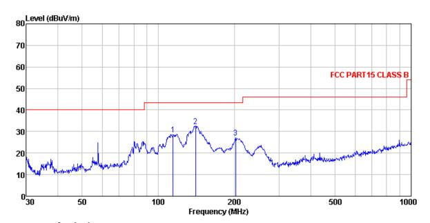
Site : 3m chamber Condition : FCC PART15 CLASS B 3m VULB9163-2013M HORIZONTAL
