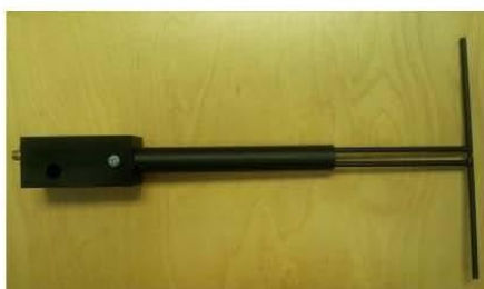
Figure 1 – MVG COMOSAR Validation Dipole
