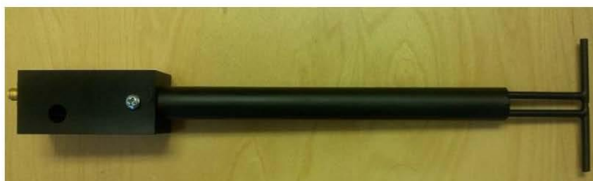
Figure 1 – MVG COMOSAR Validation Dipole
