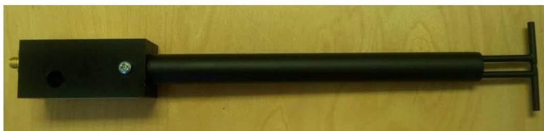
Figure 1 – MVG COMOSAR Validation Dipole
