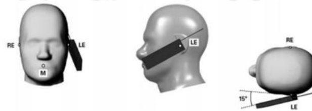
Figure 2: Tilt position of the wireless device on the left side of SAM
