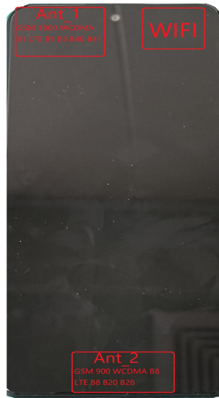
Figure 5: The location of the antennas
