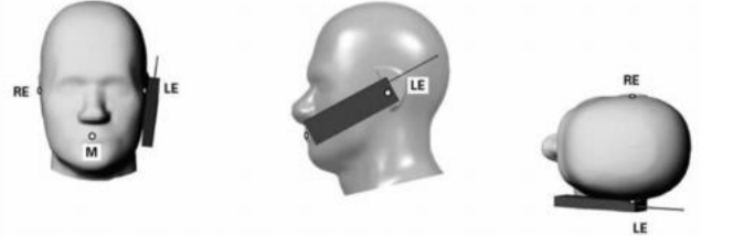
Figure 1: Cheek position of the wireless device on the left side of SAM
