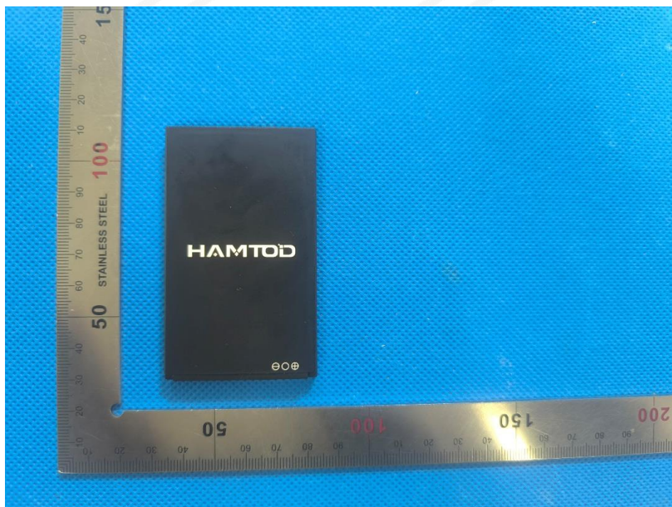
Figure 2 Back view of battery pack
