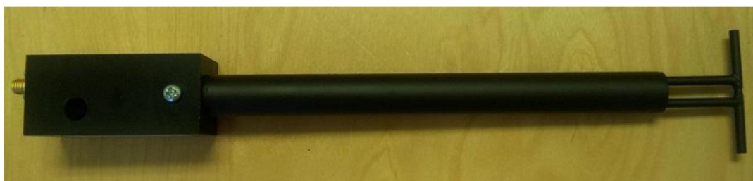
Figure 1 – MVG COMOSAR Validation Dipole
