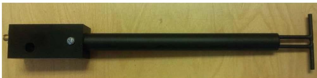
Figure 1 – MVG COMOSAR Validation Dipole
