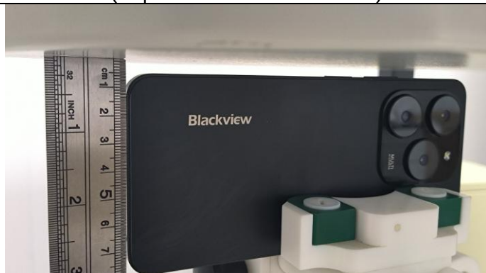
Right Side (Separation distance of 5mm)
