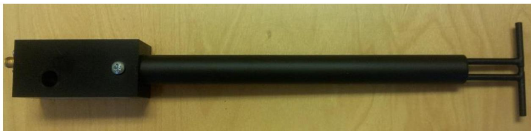
Figure 1 – MVG COMOSAR Validation Dipole
