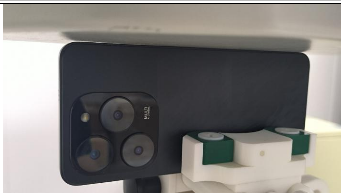
Top Side (Separation distance of 0mm)
