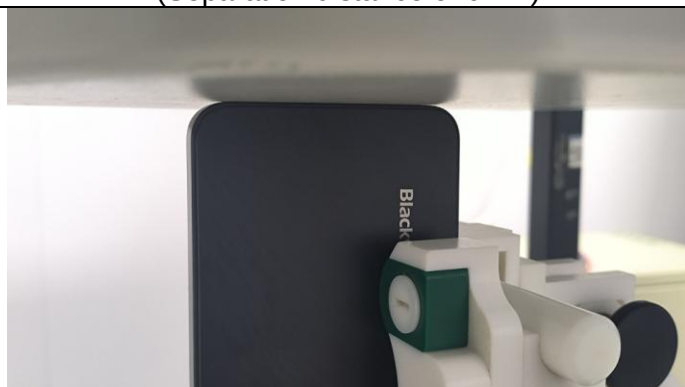
Top Side (Separation distance of 5mm)
