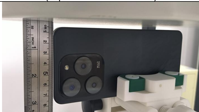
Left Side (Separation distance of 5mm)
