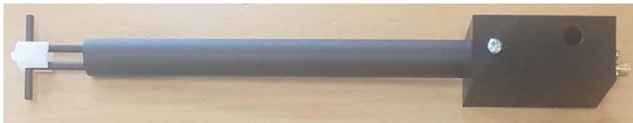
Figure 1 – MVG COMOSAR Validation Dipole
