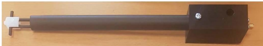
Figure 1 – MVG COMOSAR Validation Dipole
