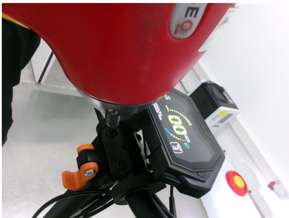
Photograph 2: Set-up of electrostatic discharge immunity test
