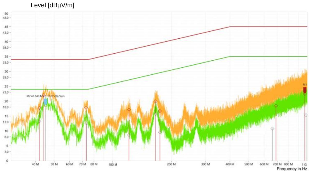
Figure 4: Spectral diagrams and measurement results, 30 – 1000 MHz, Vertical polarization, Right side
