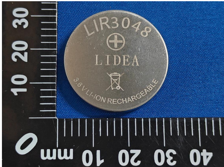
Picture 5 Front view of cell (model: LIR3048 240mAh) (Final version of the label, see main report)
