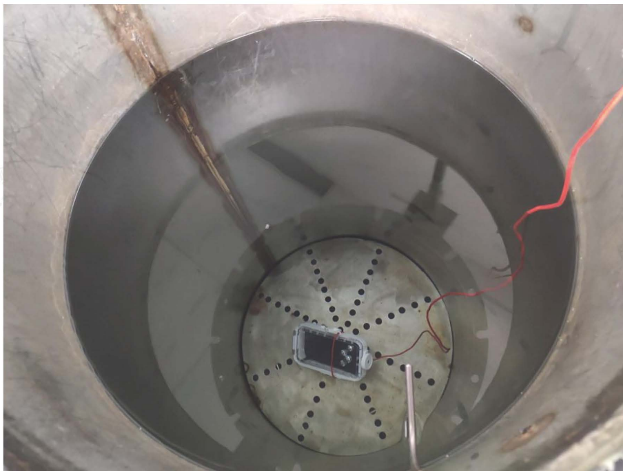
Photo 3: IPX8 test of model PU9115W
