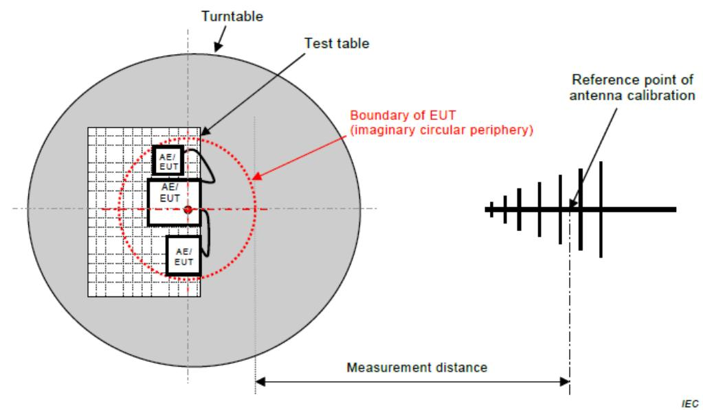
**Figure C.1 – Measurement distance**
