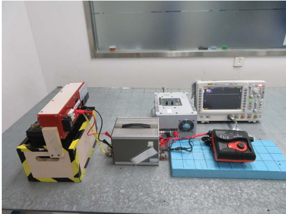
Photograph 2: Set-up for Conducted Transient Emissions from ESAs
