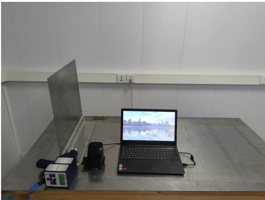
Test Setup Photo of Electrostatic Discharge Test
