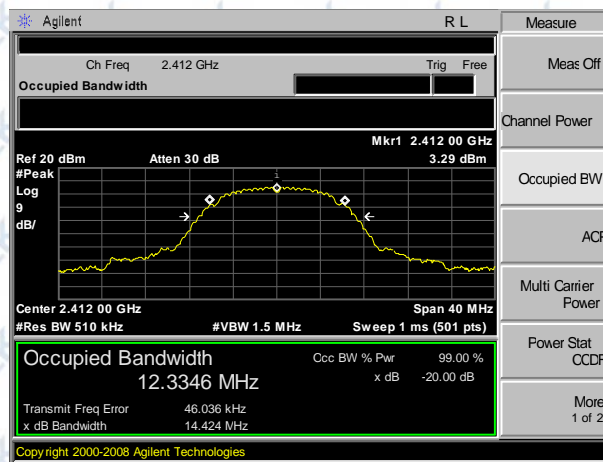
(802.11b) Measured frequencies plot on channel 1
