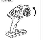
During the course of sailing forward, if you steer to the left, the tail rudder will deviate to the left and the racing yacht will turn left. With the bigger of the steering angle, the turning radius of the racing yacht becomes smaller.
