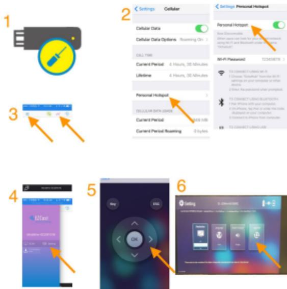
(1) Insert a paper clip into the hole on the PTVwire, and push the key inside the hole to enable HotSpot mode (Internet)
