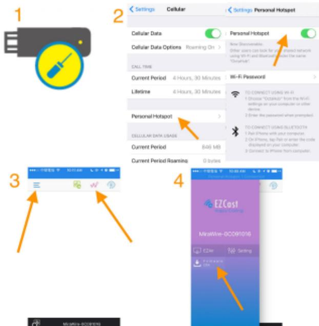
(1) Insert a paper clip into the hole on the PTVwire dongle, and push the key inside the hole to enable HotSpot mode (Internet)
