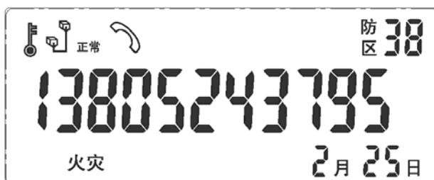
Handset icon means it is dialing alarm phone number , the digits in the middle means the phone number being called ,the date in the left corner means alarm type .
