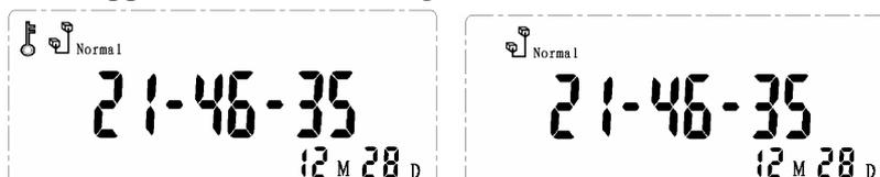
Keyboard will automatically locked when there is no any operations on the keyboard for 15 seconds.
