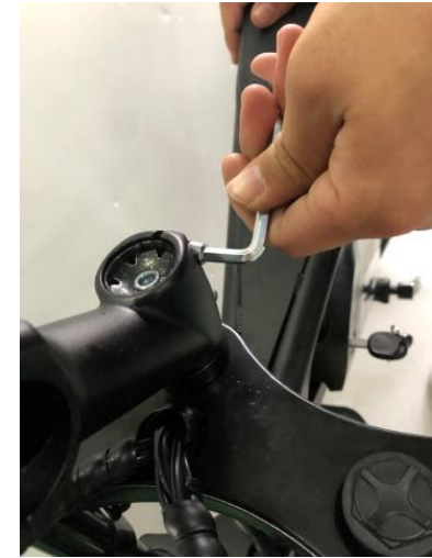
9. Slightly unscrew the screw to fix it, the handlebar holder can be moved up and down, and not too tight
