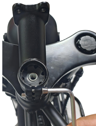
5. Use the M5 Allen wrench to unscrew the screw
