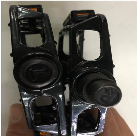
22. R for Right Pedal and L for Left Pedal
