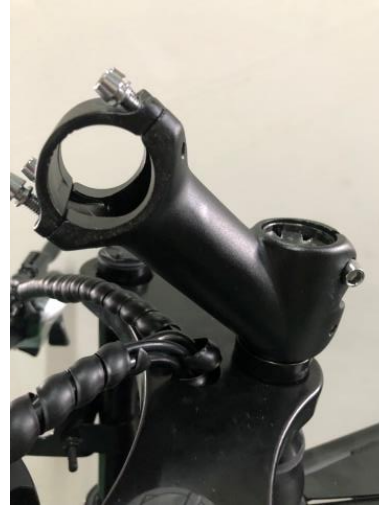
8. Adjust the direction of the handle holder so that it faces the front
