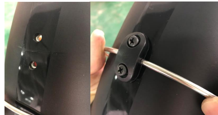
30. Put the rear fender bracket into the buckle, as shown in the picture, tighten the screws
