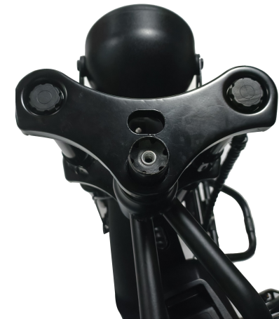
6. Unscrew the screw and remove the trim cover
