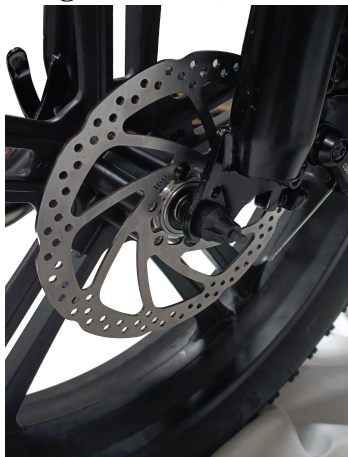
19. Take out the disc brake from the tool box and install it on the front wheel, then insert the front wheel into the front fork slot
