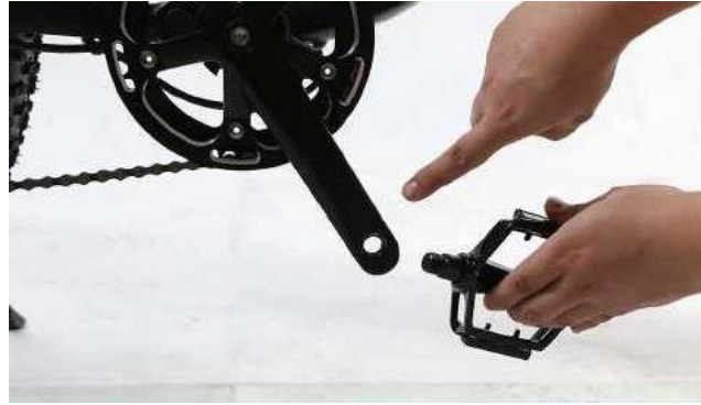
23. Insert the pedal(s) into this position
