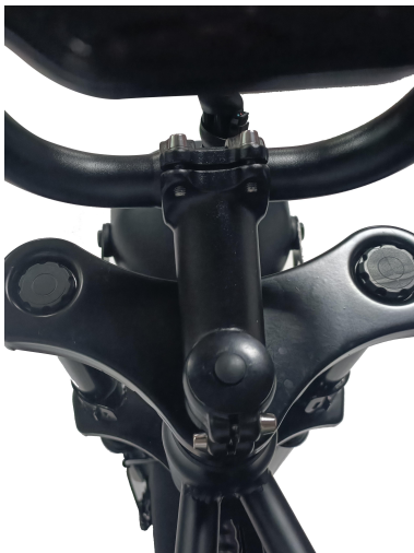
4. Pull off the silicone protective cover on the top of front fork
