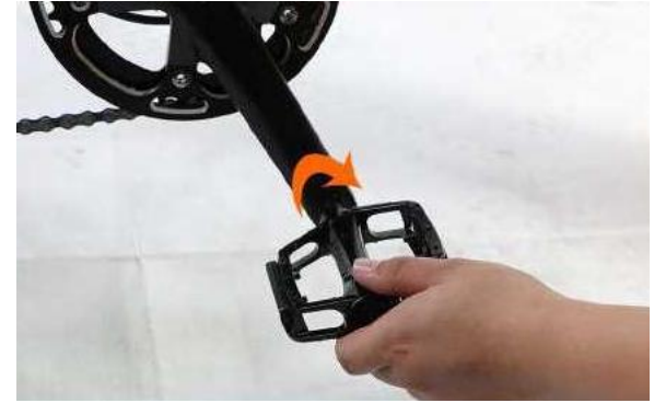
24. Slightly secure the pedals into the crank arms in a clockwise direction
