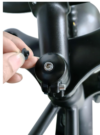
11. Tighten the screws with an M5 Allen wrench to make the front fork fit closely with the frame, and there should be no gaps and no shake.
