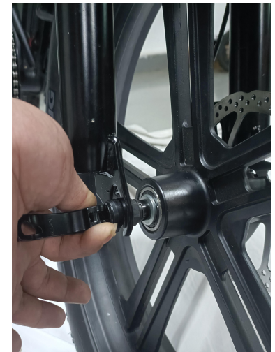
21. Tighten it with the 12-14 wrenches until it is not loose.
