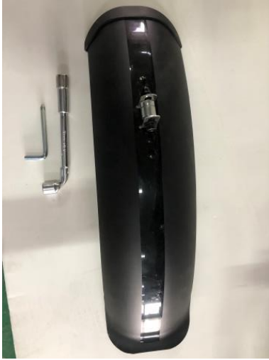
16. Take out the front fender and M5 Allen wrench and socket wrench from the tooling kit
