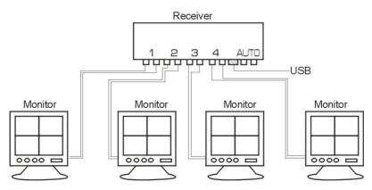
4. Connect the receiver to one monitor to see one picture one time, press the channel switch keys on the receiver, to get the picture form right channel, or press AUTO key to see 4 piectures by anto change.
