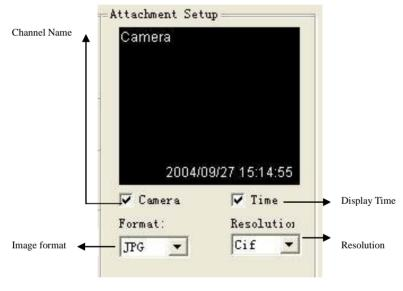
Fig 4.19 Attachment Setup
