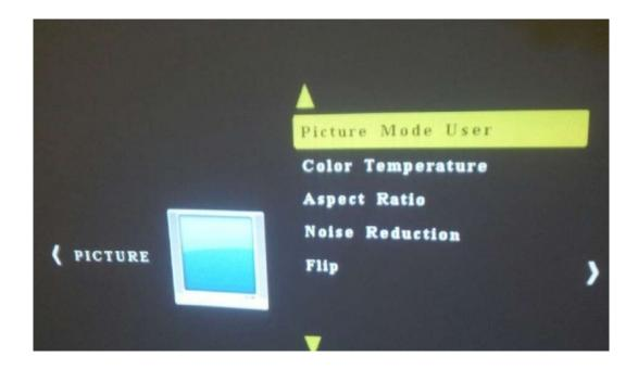
Select the options to be regulated and press OK to enter. Then press V+ or V- to regulate. To regulate contrast ratio, press to choose the option of contrast ratio.
