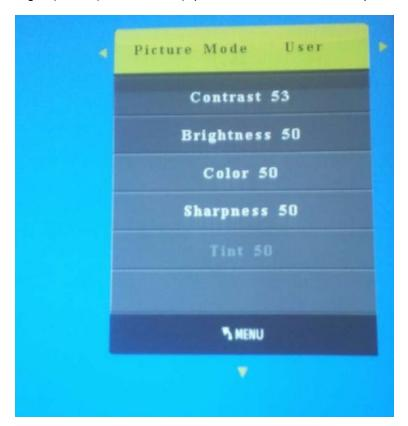
Press P- to select options to be regulated and then press V+ or V- to regulate. Press the option of luminance to regulate image luminance.
