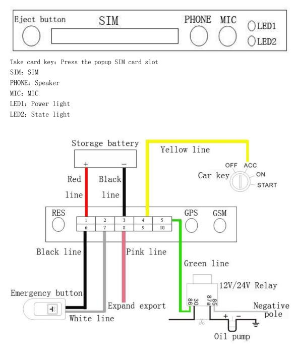
RES: Reset GPS: GP S Antenna interface GSM: GSM Antenna interface 2、8、9、10: Expand interface
