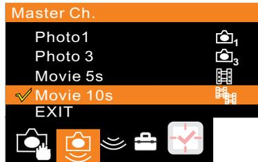
**Photo 1:** Snap shot 1 photo when motion detected
