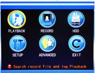
Note: The setup of all the submenus below will not be effective until "Enter" is pressed. The setup of this menu will be invalid if you exit directly. A significant characteristic of this product is when you move the cursor to any option, the prompting message of this option will be displayed automatically in the lower part of the screen.
