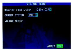
**VGA resolution:** Left-click or press "Enter" to set the VGA output resolution, with the 3 options of 1280\*1024, 1024\*768 and 800\*600;
