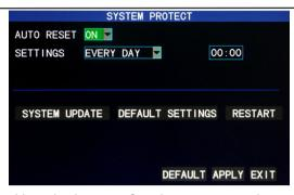
**Auto reset:** When this option is set to "On", the user can set the restart frequency and time of this device himself/herself.
