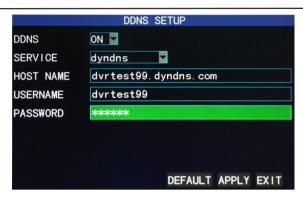
**DDNS** (domain name resolution): with the two options of "Enable" and "Disable"; when a domain name resolution server is available, please select DDNS Enable;
