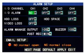
I/O state alarm: Each channel corresponds to an I/O state alarm, i.e., when the alarm input of a channel is valid, the alarm record of the corresponding channel will be started.
