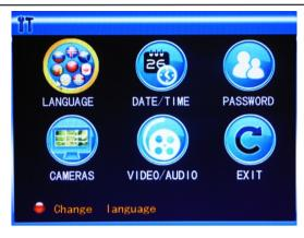
The Basic Setup screen includes the 6 options of System Language, Time Setup, User Password, Display Setup, Video/Audio Setup and Exit.
