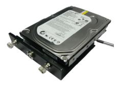
2 Connect the hard disk data cable well, put the hard disk into host
