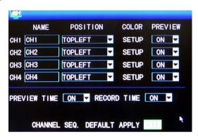
**Channel name:** Move the cursor to the input box of this option, and press "Enter" to enter the input screen of this option. Numerical, English and Chinese pinyin input methods are supported;
