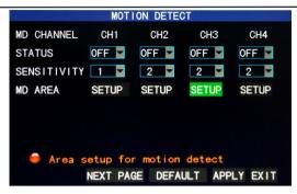
Channel switch: Each channel has a corresponding switch. Press "Enter" to select motion detection "On" or "Off".
