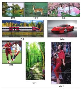
Kind reminder: Press the corresponding stitching button on the machine MODE or remote control to achieve various image stitching efects, such as 1X1, 1X2, 1X3, 1X4, 2X2, 2X1, 3X1, 4X1 (row X column)
