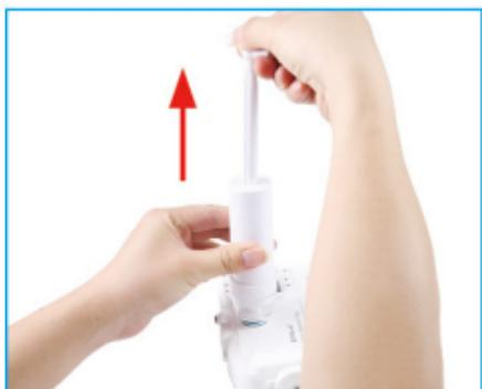
5. Use the pump to pump up the vacuum, the installation is complete.
